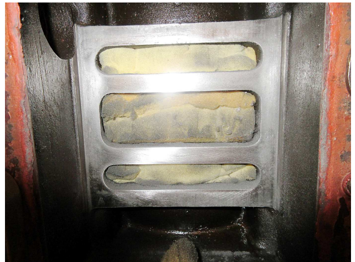
The engine cylinder port face now all flat with no ridges
