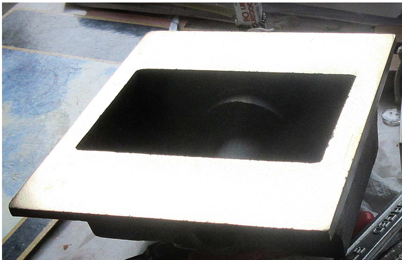
The engine slide valve now with a lovely shiny flat surface
