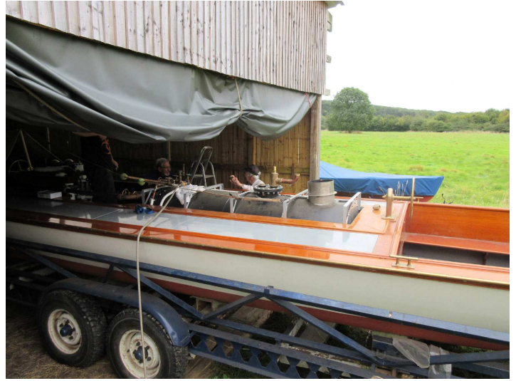
Filling the boiler with water via the hose
