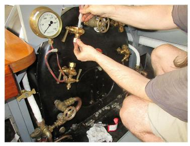
Photos above show the fitting of the boiler water gauge cocks and lining up ready to insert the gauge glass tube. The holes in the backhead are 3/4" BSP which needed cleaning before installing and sealing in position. We had not fitted these earlier to avoid exposure to damp air and losing their nice polished finish.
