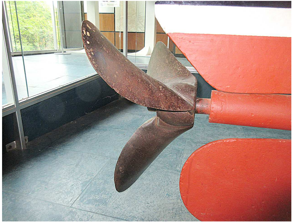
Photo taken before museum closed. Note rudder is in front of the propeller, typical of many small Victorian vessels
